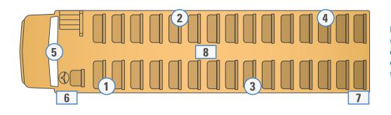
Record four, six or eight channels (based on your recorder of choice). Determine your channel count and camera locations for the level of coverage you need.
